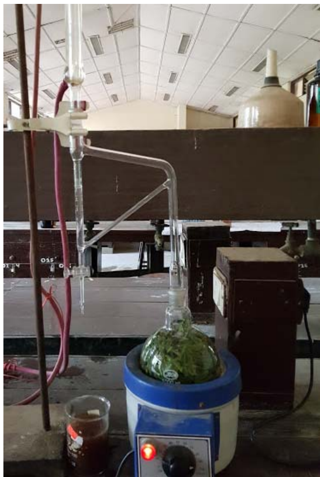
Plate 1: Hydrodistillation of 200 gram of lemongrass leaves in 500 ml of water
