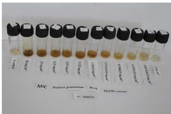
Plate 3: Determination of minimum inhibitory concentration (MIC) of methanolic bark extract of Punica granatum L. against MRSA
