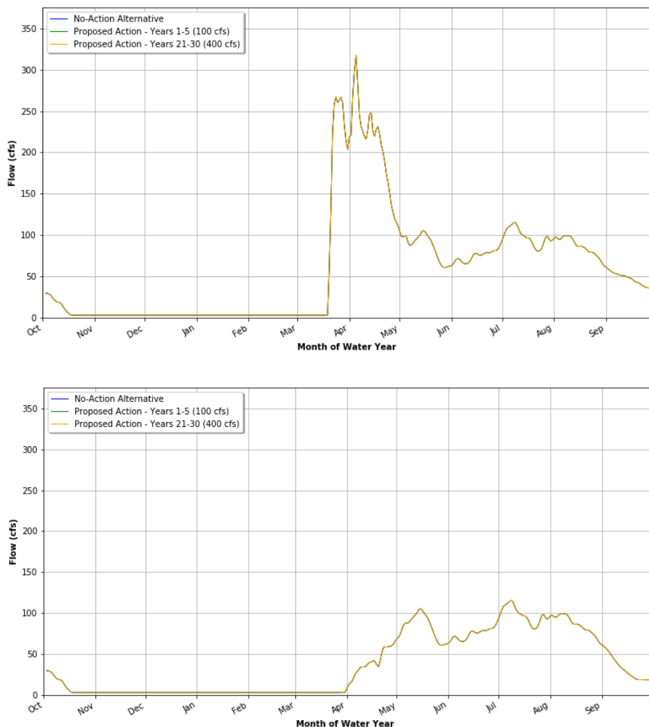
Figure 54. The Ochoco Creek Hydrograph for the No-Action Alternative and Proposed Action in Years 1–5 and 21–30 in Representative Normal (top) and Dry (bottom) Years at the OCHO Gauge
