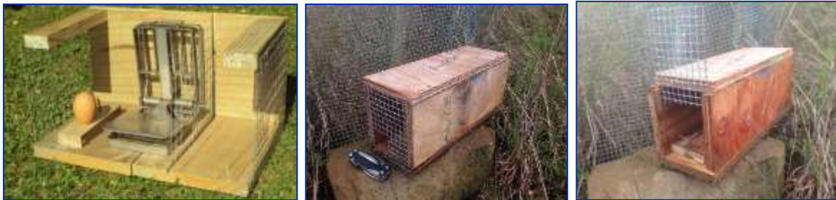
Figure 11.1. Bird Excluding Box for DOC 200 Snap Traps from Makamaka'ole Project, Maui
