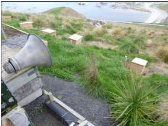
Figure 11.3. Social attraction speaker system and nest boxes at Hutton's shearwater colony, Kaikoura, New Zealand. A. Raine
