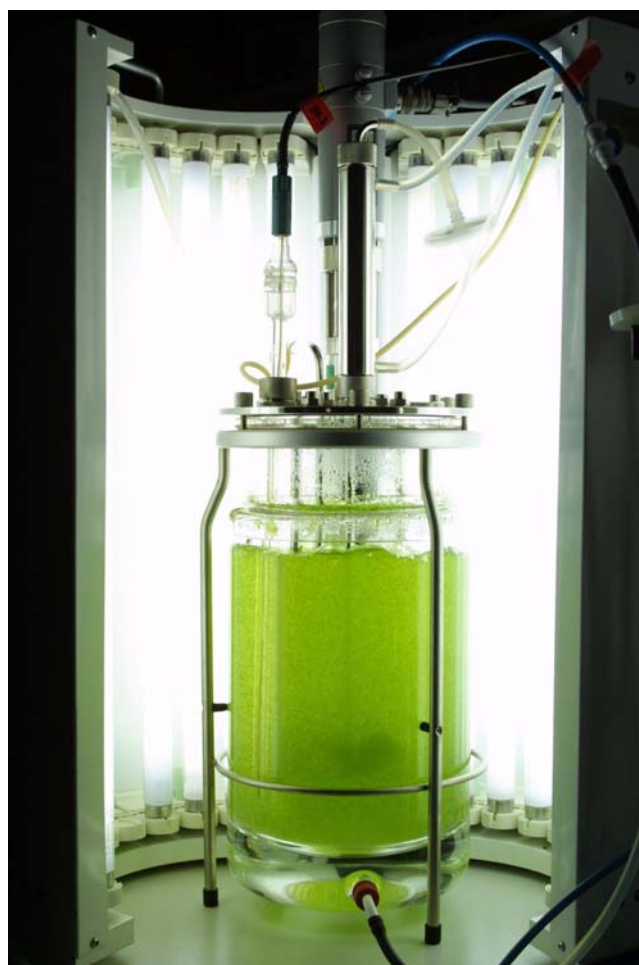
Figure 97. This type of bioreactor is used to grow Physcomitrella patens for human proteins and human blood-clotting factor IX. Photo by Ralf Reski.
