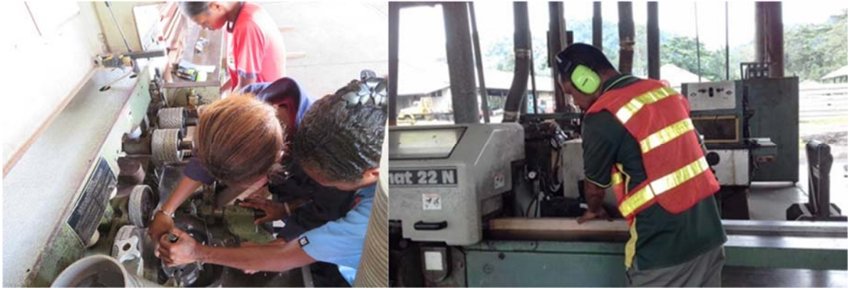
Figure 5. Setting up of planer moulder (left) and planing trials (right) (Photos: Ravu Iru).
