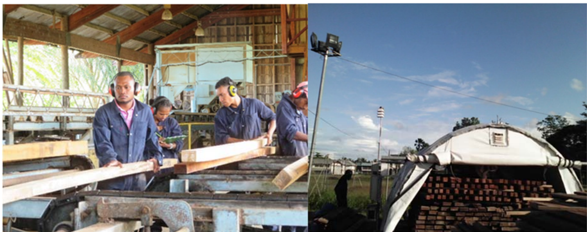
Figure 4. Timber milling at TFTC (left) and solar drying at PNG Unitech (right) (Photos: Ravu Iru).
