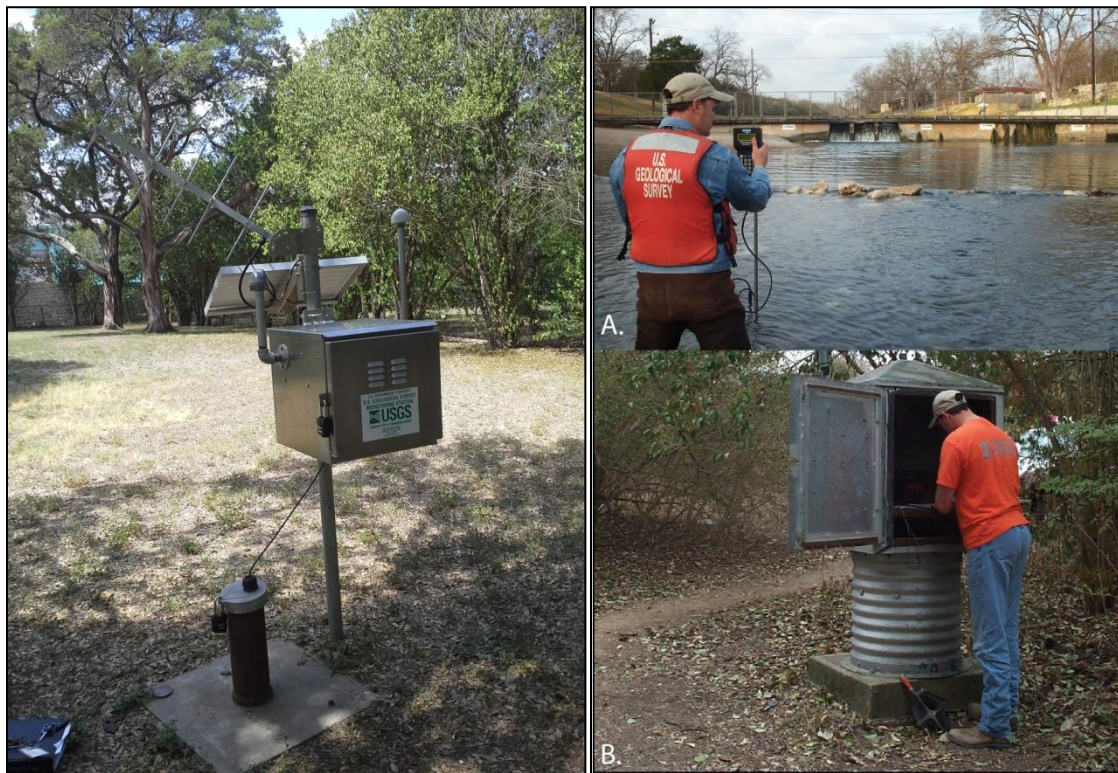
(Left) Photograph of the Lovelady (58-50-301) well with U.S. Geological Survey equipment. The USGS took over continuous monitoring in August 2013. The USGS site name and number is 301237097464801 YD-58-50-301 (Lovelady). (Right) A) Photograph of USGS staff measuring flow about 250 ft downstream of Barton Springs Pool dam using a FlowTracker ADV®. Note the rock wall creating turbulence. B) USGS staff check equipment and make a manual stage measurement in the USGS Barton Well. More information on the Barton Springs discharge methods are discussed in Hunt et al., 2012.
