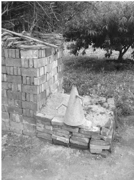
FIGURE 6.10 Unusual condenser system and commonly used receiving can (oil separator) used in cornmint oil distillation in China.
