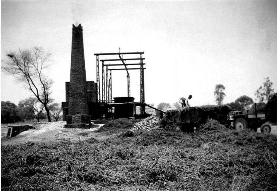
FIGURE 4.11 A field view of the larger-sized multiple tank unit installed in a big mint farm in India. This unit is for four tanks. Semidried mint herbage is unloaded from a tractor trolley. It is spread around to allow further loss of moisture.
