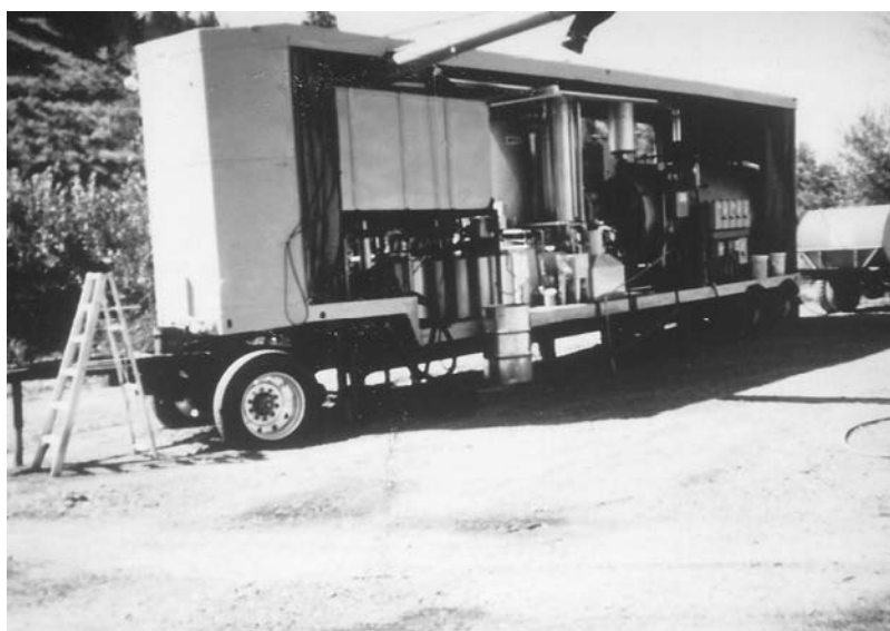
FIGURE 6.6 Example of mobile distillery designed by Newhouse Manufacturing, Inc.
