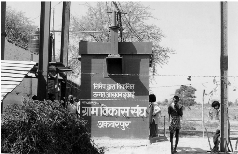
FIGURE 4.12 Mint herbage distillation unit designed by CIMAP, Lucknow, installed for cooperative use in a village in Barabanki district of Uttar Pradesh in India.
