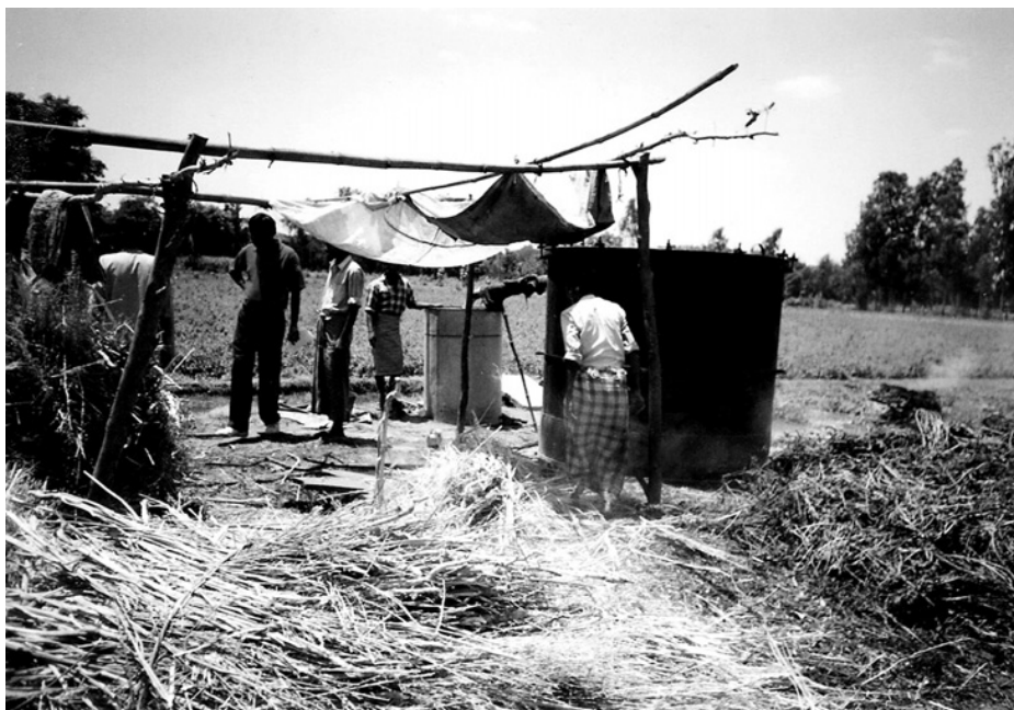
FIGURE 4.10 A water-cum-steam distillation unit of the kind fabricated in Indian villages used in a mint field. The agrowaste to be used as fuel and dry herbage to be distilled are also seen.
