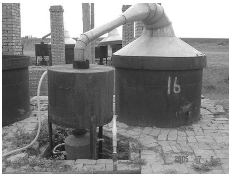
FIGURE 5.2 A single distillation unit in Anhui Province showing the condenser tank which houses a spiral tube condenser and receiver.
