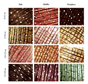
Figure 7. Microscopic features of the Pterygota alata vessels with pith, middle and periphery section with different girth classes (magnification 4x)
