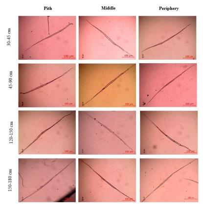
*Figure 6. Microscopic features of the Pterygota alata fibres with pith, middle and periphery section with different girth classes (magnification 10x)*
