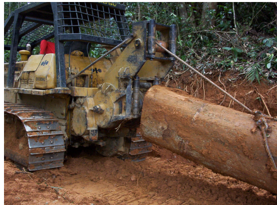
Fig. 4. The front-end of the log is lifted off the ground during skidding operation.
