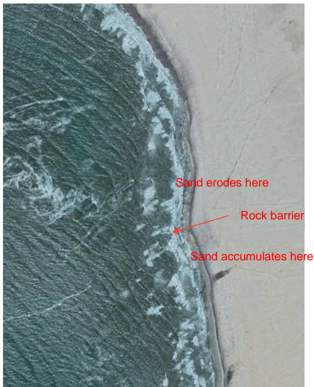
Figure 2-6: Rock barrier inducing sand accretion and erosion to form a kink/bump in the shoreline at Wlotzkasbaken.
