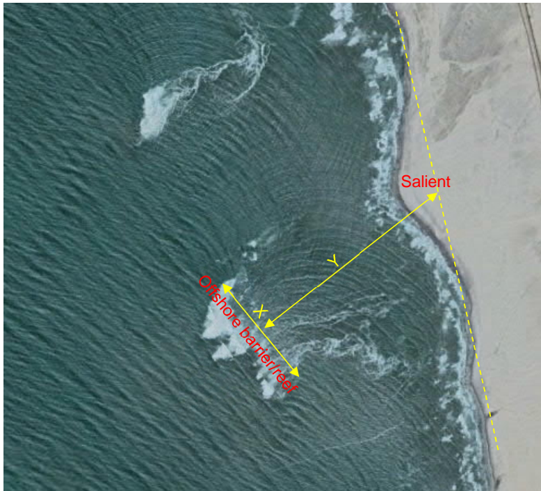
Figure 2-7: Salient formation at Wlotzkasbaken
