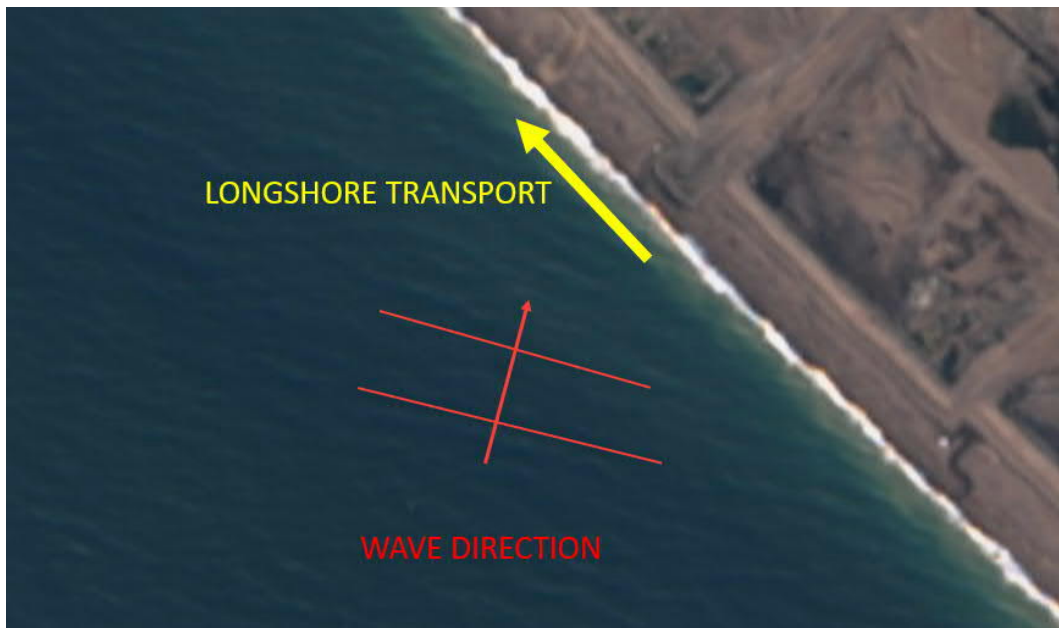
Figure 2-5: Longshore transport driven by obliquely approaching waves.
