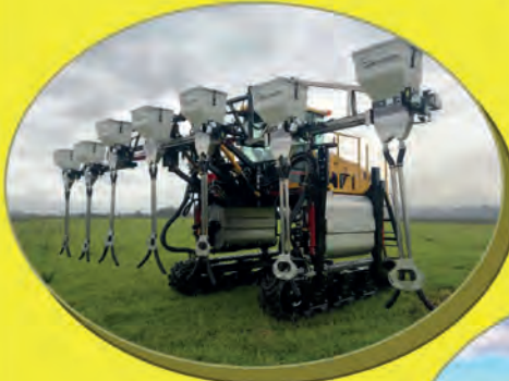
TR6 SPRAYER Over-the-Row wet/granular system
