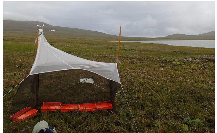
Figure 2: Malaise-Flight Intercept Trap hybrid near the NW coast of St. Matthew.
