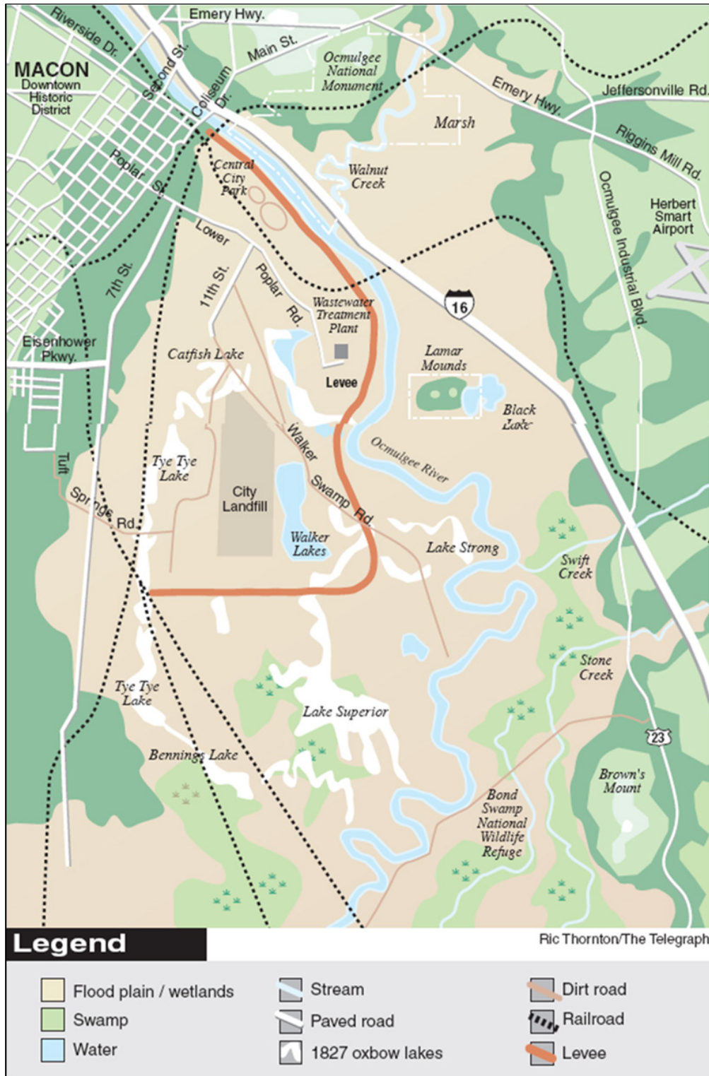
Figure 22. Map showing present-day general features of the Ocmulgee River floodplain near Ocmulgee. Note the meandering channel below the Macon levee, vs. the channelized river in the Ocmulgee area. Other features include the City of Macon landfill across from the Lamar Unit, and the Macon water pollution control plant, which discharges 0.29 kilometer (0.18 mi) below the Lamar Unit. Map by R. Thornton, with permission from The Telegraph.
