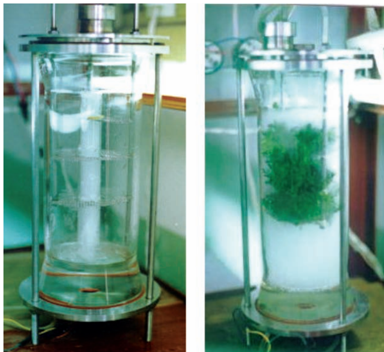
Fig. 23.4 A nutrient mist bioreactor for artemisinin production from A. annua L. shoot cultures.
