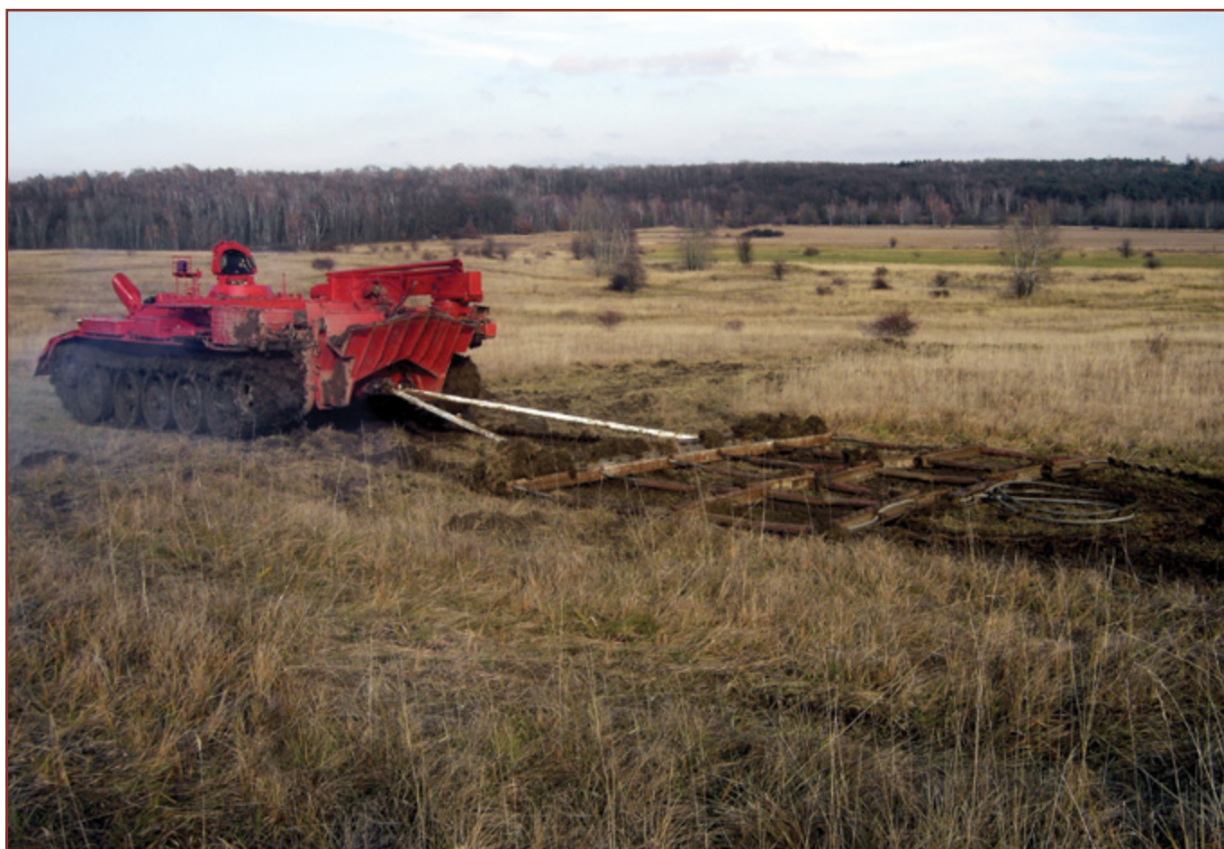
Fig. 1. One of the methods used for mechanical vegetation disturbances. A set of rails can only be dragged with a tank. (P. Vaňhát)
